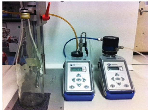
Fig. 11: Sample is taken by a Beverage Package Sampler (left), transferred to Orbisphere 3650 (center) and then to Orbisphere 3658 (right)
