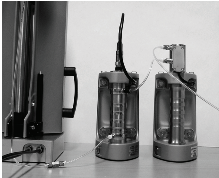
Fig. 9: Set-up for the simultaneous measurement of O 2 and CO 2 with the connection in series PFD Filling Device (left), OxyQC (center) and CarboQC (right) (image: Anton Paar GmbH)
